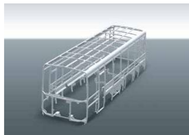
Lightweight aluminique alloy frame
