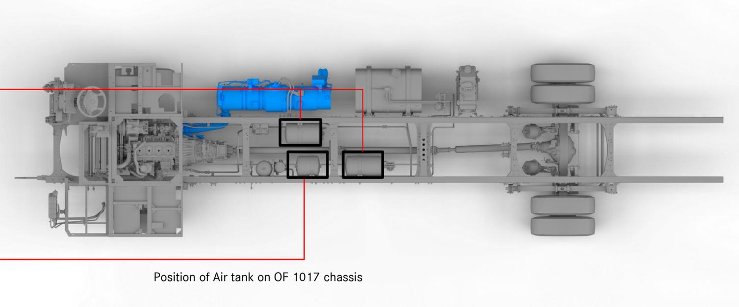
Position of Air tank on OF 1017 chassis
