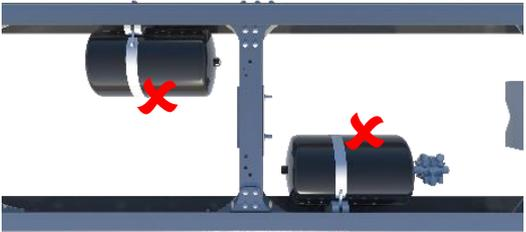
Position of compressed air tank for Service Brakes
