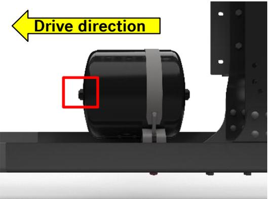
Auxiliary tank B42.00-1010-01 Position of auxiliary tank on the chassis, suitable for additional pneumatic connections
