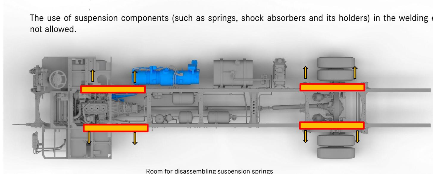
Check the possibility of disassembling the front and rear suspension springs, as shown in the figure.
