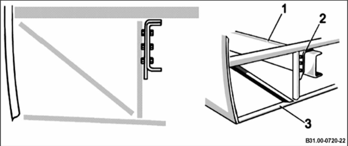
Body fastening by means of corner plates
