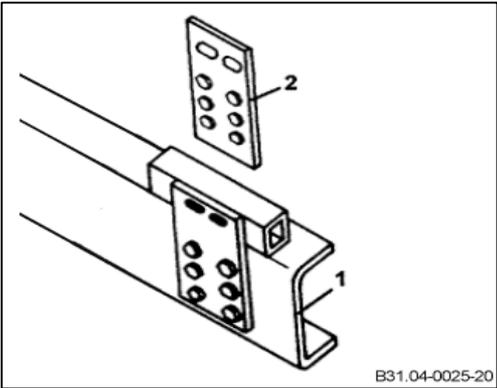
Body fastening by means of corner plates
