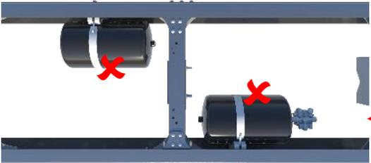
Position of compressed air tank for Service Brakes Not suitable for additional pneumatic connections
