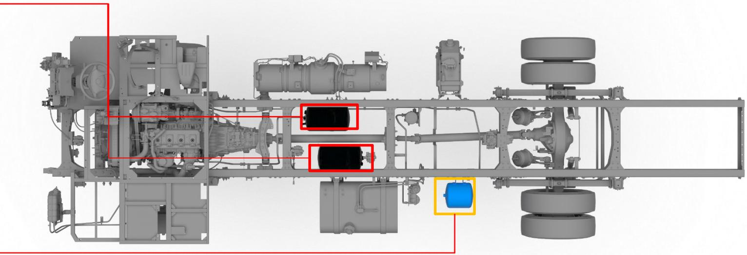
Position of Air tank on OF917 4250WB chassis
