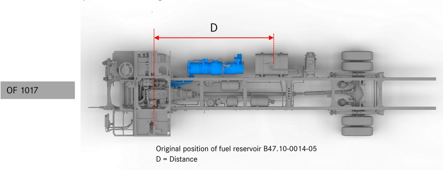
**Tab8- Original fuel tank position for OF 1017**
