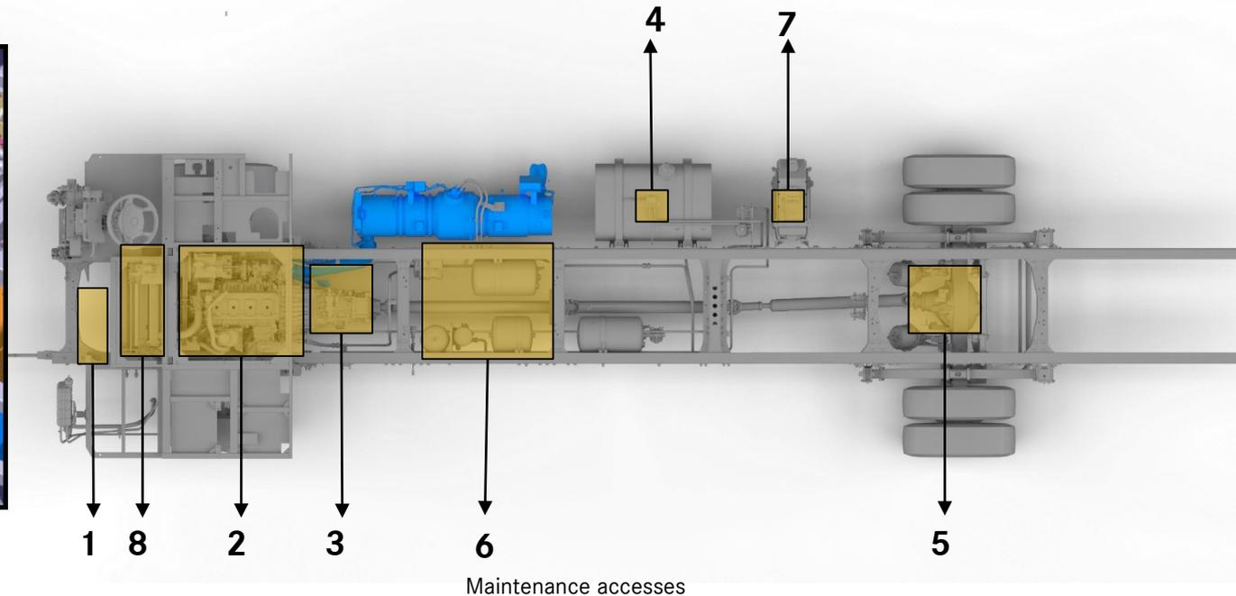
1. Access to the expansion tank upper part, hydraulic steering oil reservoir, clutch fluid reservoir, instrument cluster;
