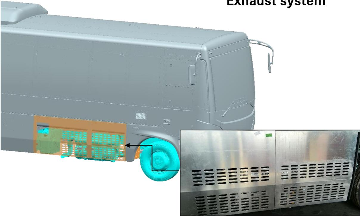
Clearance of Min 50mm to be maintained above the ATS area
