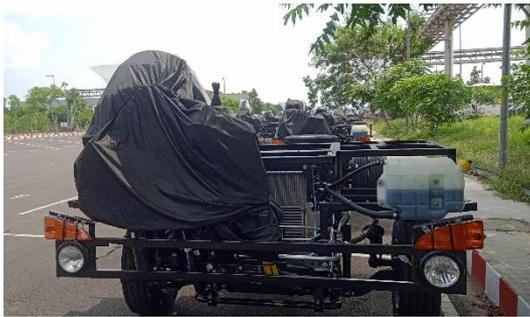
Plastic protective cover for Instrument panel and Electrical & electronic components
