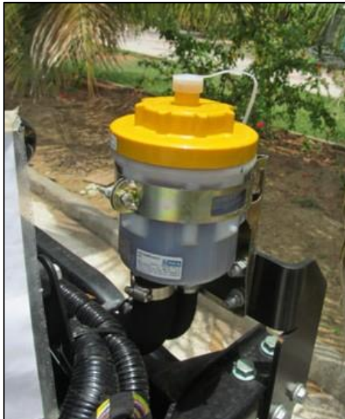
Power steering oil tank
